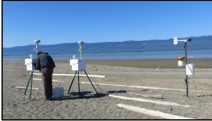
FIGURE 3.7. DEPLOYMENT OF THE BGI PQ200 PM 10 AND PM 2.5 SAMPLERS AS WELL AS THE ASSOCIATED METEOROLOGICAL INSTRUMENTATION AT CHOWIKA BEACH.
