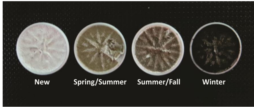
FIGURE. 4.5. REPRESENTATIVE FILTERS FROM THE TSAY KEY TEAM THAT WERE COLLECTING PARTICLES <2.5 \mu\text{m} FOR DIFFERENT PERIODS OF THE YEAR.
