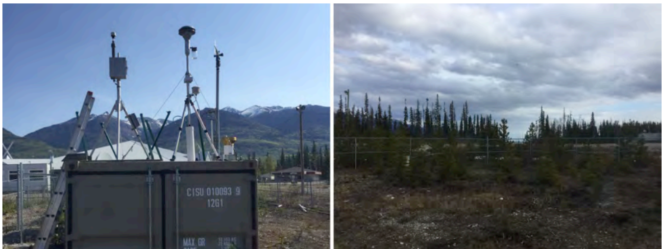
Figure 2: Regional Monitoring Network site and Reference Station within Tsay Keh Dene. E-Sampler atop the TEOM enclosure on the left (next to a ladder) and TEOM inlet on the right. The right image is facing towards the southeast and the reservoir.
