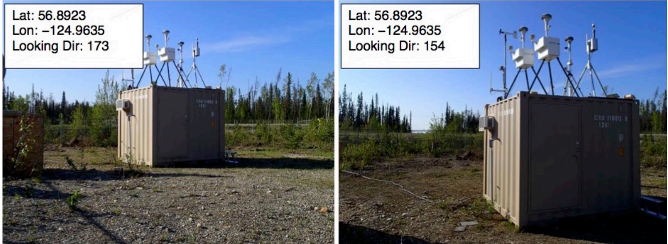
Figure 12: Tsay Keh Dene Regional Monitoring Network and Reference Station – E-Sampler is on top of enclosure.
