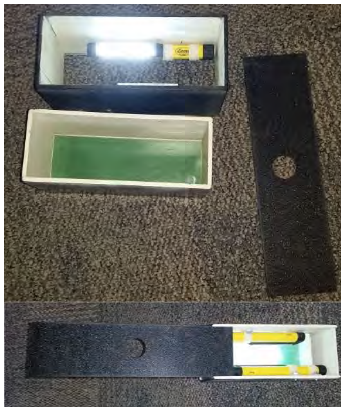
Figure 4. The amphibian camera box disassembled (top panel) and assembled (bottom panel).
