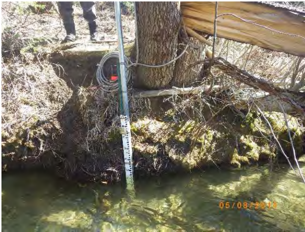
Photo 1. Gauging station on Six Mile Creek with temperature probe installed.
