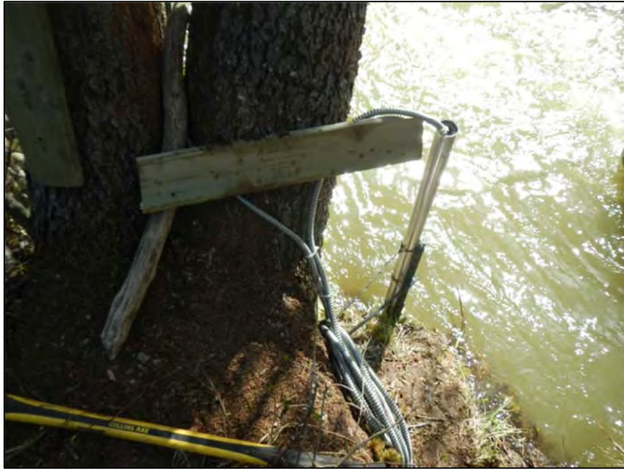
Photograph 1: Housing for water level and temperature probe at Six Mile Creek gauging station.
