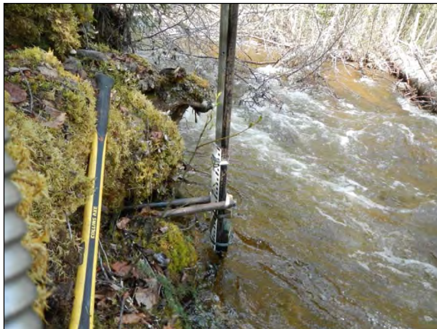
Photograph 2: Housing for water level and temperature probe at Ole Creek gauging station.
