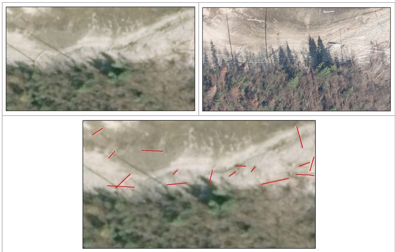
Figure 3-1 Example of the analysis of faint details on the imagery of 2009, by using the new set of 2011 to confirm the existence of woody debris
