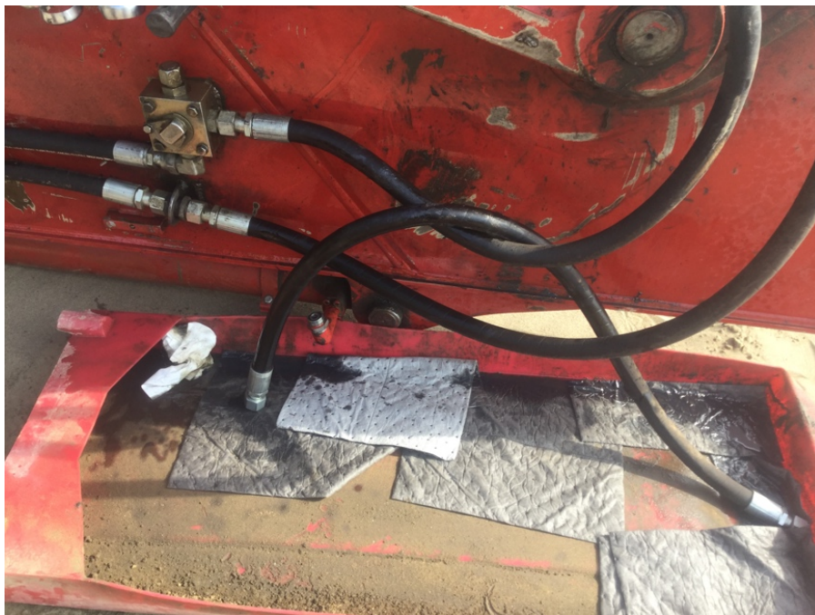
Figure 15: Managing and replacing leaking hoses with spill kit and tray.
