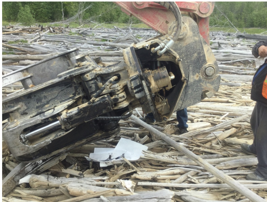
Figure 14: Grapple implement in resting position during repair with spill pads below.
