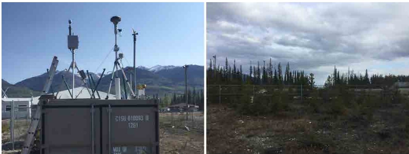
Figure 2: Tsay Keh Dene Regional Monitoring Network and Reference Station. The E-Sampler is atop the TEOM enclosure (TEOM inlet is to the right of the E-Sampler). The image on the right is facing towards the southeast.
