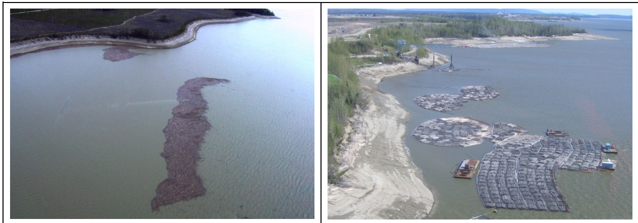
Figure A-3 Large floating debris (F3) and log booms (FO) managed during the cleaning program
