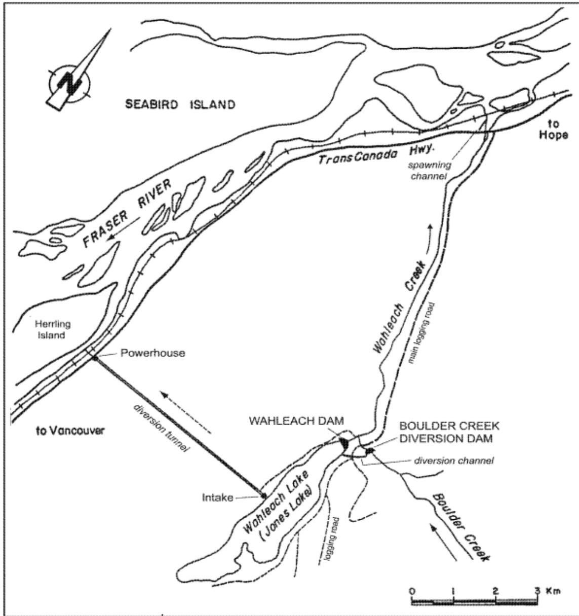
**Figure 1. Location and general arrangement of the Wahleach Diversion Project.**
