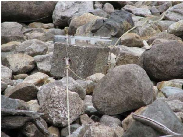
**Figure 2.8: Littoral Sampling Apparatus (Cement Block and Buoyant Tray) (Pre-2011)**
