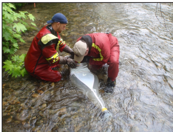
Photo A18: Hess Sampler being churned over 20 times with trowel.
