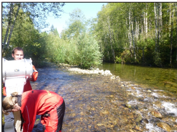
Photo A 19: Rinsing mesh tunnel between samples (Site 6 downstream September 2014).
