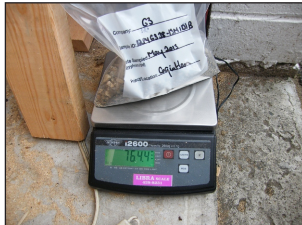
Photo A 26: Subsurface <10 mm sample weighed before sending to laboratory for particle size analysis (October 2013).
