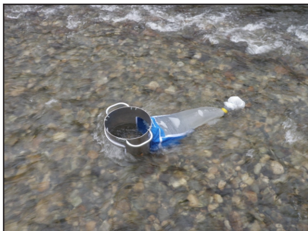
Photo A9: Hess Sampler in river substrate, facing upstream to aid flushing of fines from sample into downstream funnel
