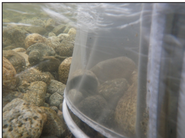
Photo A13: Modified Hess Sampler with 20 micron mesh to prevent loss of fine particles
