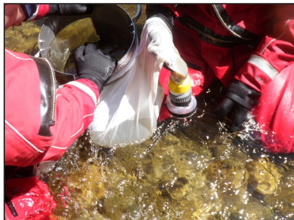
Photo A14: Surface sediment flushed and collected into a 20 \mu m filter
