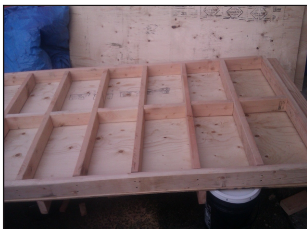
Photo A17: Drying rack used to prepare sample for sieving
