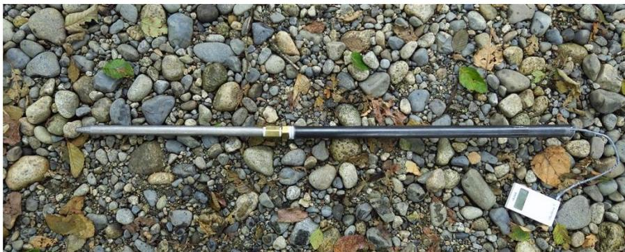
Figure 2. Hyporheic temperature probe used to measure water temperature 25 to 30 cm into substrate.
