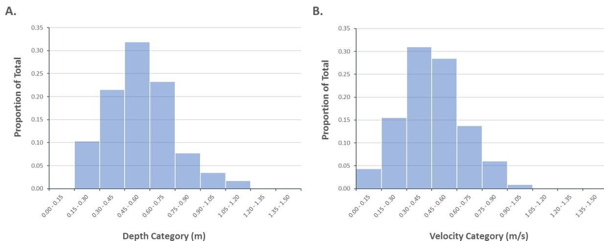
Figure 9. Water depth (A) and average velocity (B) habitat-use frequency histograms for Coho Salmon spawners. Based on 116 paired observations at redd sites collected over a 4-year period (2008 - 2011). Sampling dates and average daily discharge at the time of sampling are provided in Table 6.
