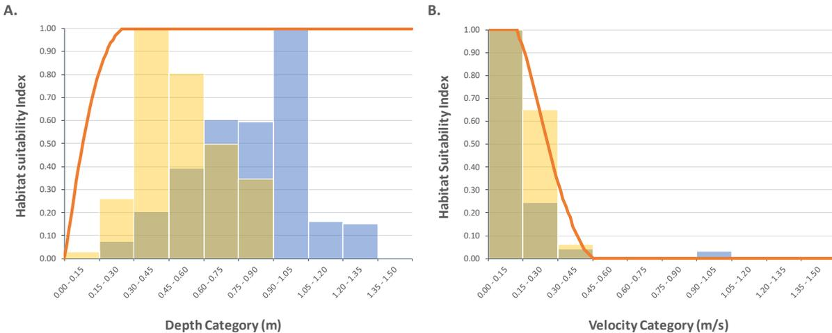
Figure 36. Comparison of generic (red line) and stream-specific (histogram) HSI functions describing depth and velocity preferences for Coho fry. The Pre-WUP HSI functions are in blue, WUP in gold.
