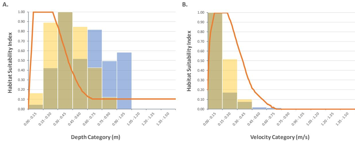
Figure 34. Comparison of generic (red line) and stream-specific (histogram) HSI functions describing depth and velocity preferences for Steelhead fry. The Pre-WUP HSI functions are in blue, WUP in gold.
