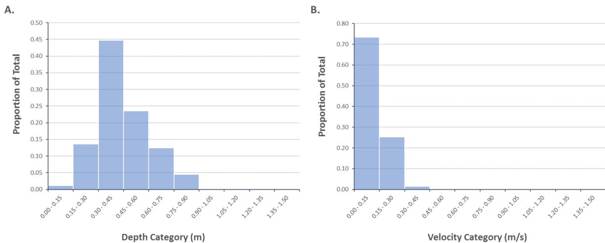
Figure 23. Water depth (A) and average velocity (B) frequency histograms illustrating habitat-use of Coho fry following WUP implementation. Based on 353 depth/velocity observations collected over a 3-year period (2009 – 2011). Sampling dates, site locations and discharge at the time of survey is provided in Table 7.
