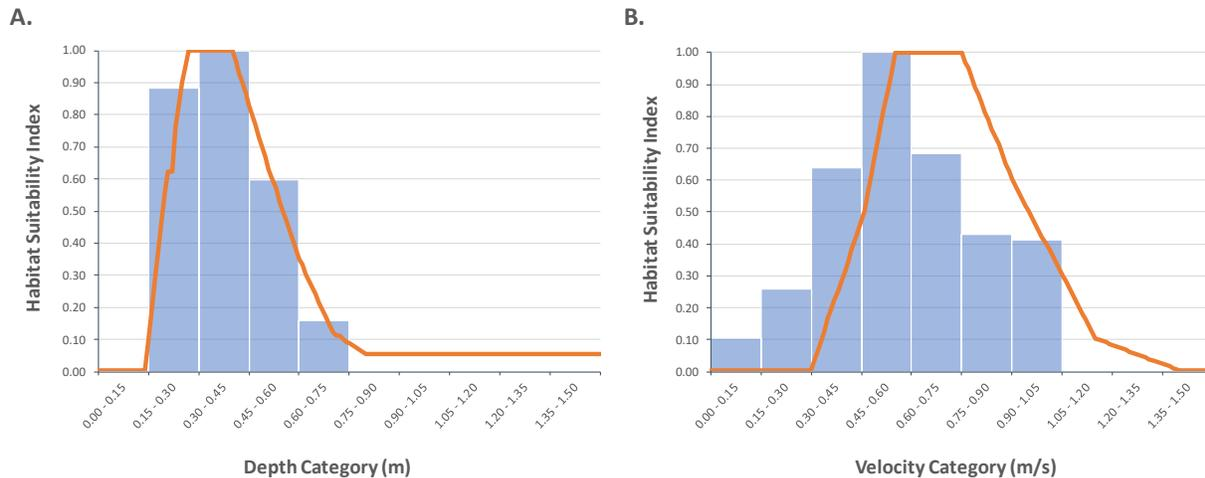
Figure 33. Comparison of generic (red line) and stream-specific (histogram) HSI functions describing depth and velocity preferences for Chum spawners.
