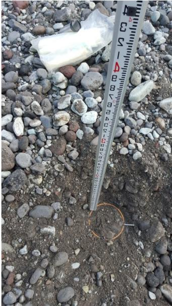
**Photo 3: Sediment trap in bar top at Eagle Point also buried under ~30 cm of sediment following Jan. 2016 discharge event.**
