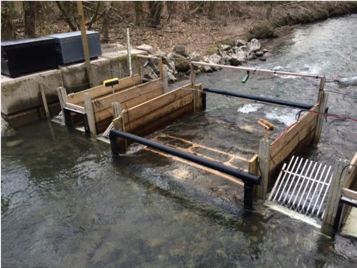
**Figure 5. Downstream photo of the NVOS counter site showing the new middle channel made up of two directional antennas (one upstream and one downstream) and a resistivity counter pad**
