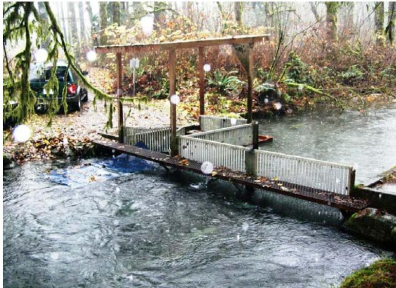
**Figure 6:** Tenderfoot Creek enumeration site. Pre-spawners pass into a vee-type trap box before becoming manually counted by DFO staff.
