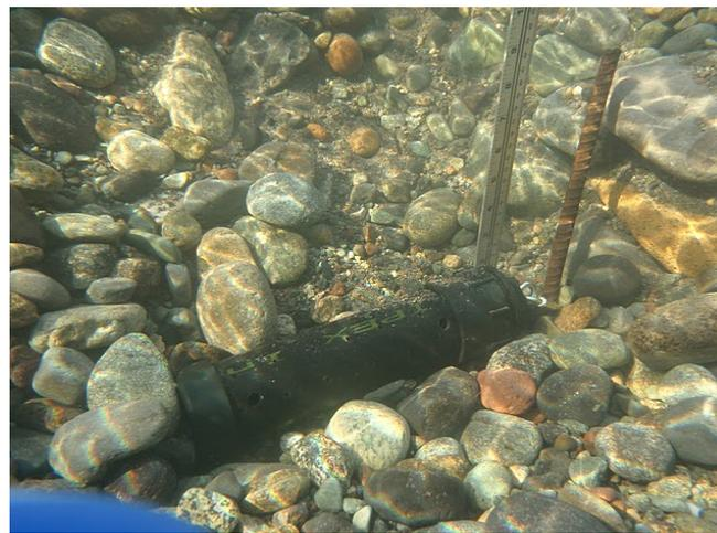
**Figure 8:** TOP – water temperature logger becomes incorporated into a capped 30cm section of perforated PVC pipe to form a simulated egg capsule. BOTTOM – one of nine capsules is anchored and then 6 reburied into randomly selected chum redds near Moody's Beach and 3 at the Gauge Pool.
