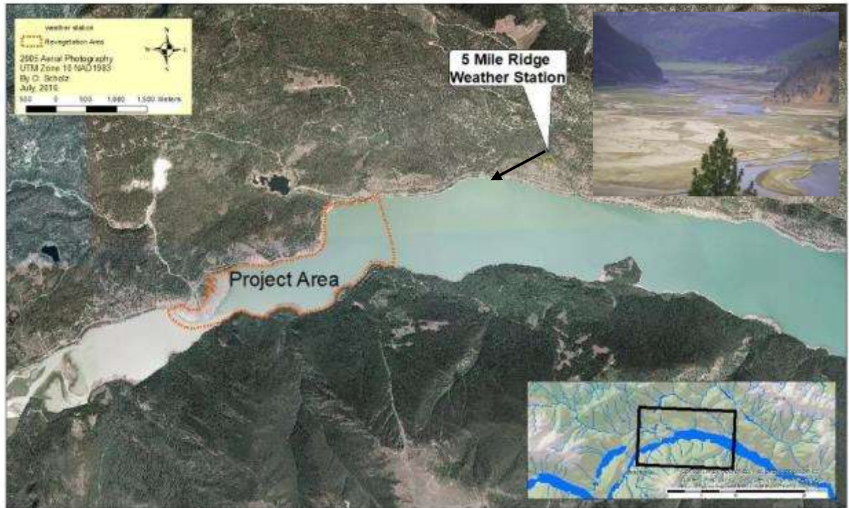
Figure 7. Map showing location of the dust storm monitoring weather station with cameras orientation relative to project area. Example of station photo inset.
