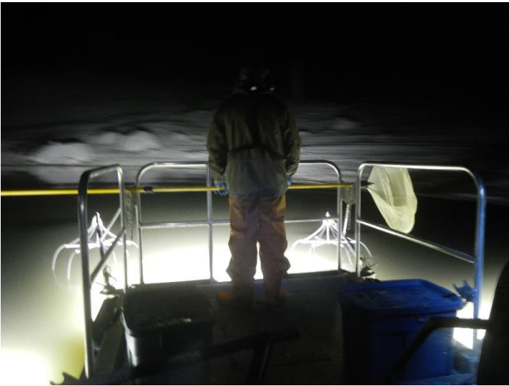
Plate 2 Boat EF is conducted by running an electrical current through the water between a set of boom-mounted anodes extended off the front of the boat and a cathode array, while propelling the boat forward at slow speed.
