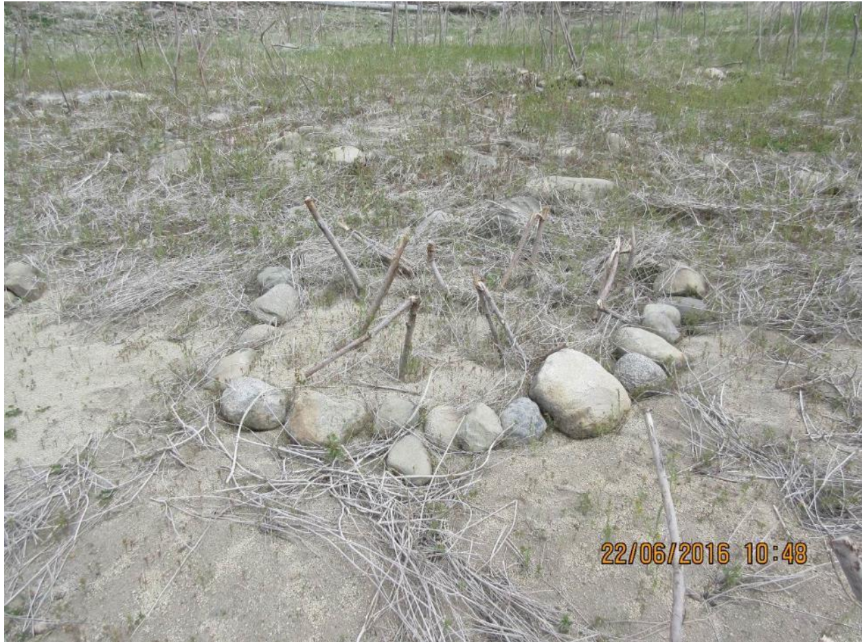
Figure 20. Example of the mechanical damage from ice on live-stake cuttings planted in 2015 (STB terrain).
