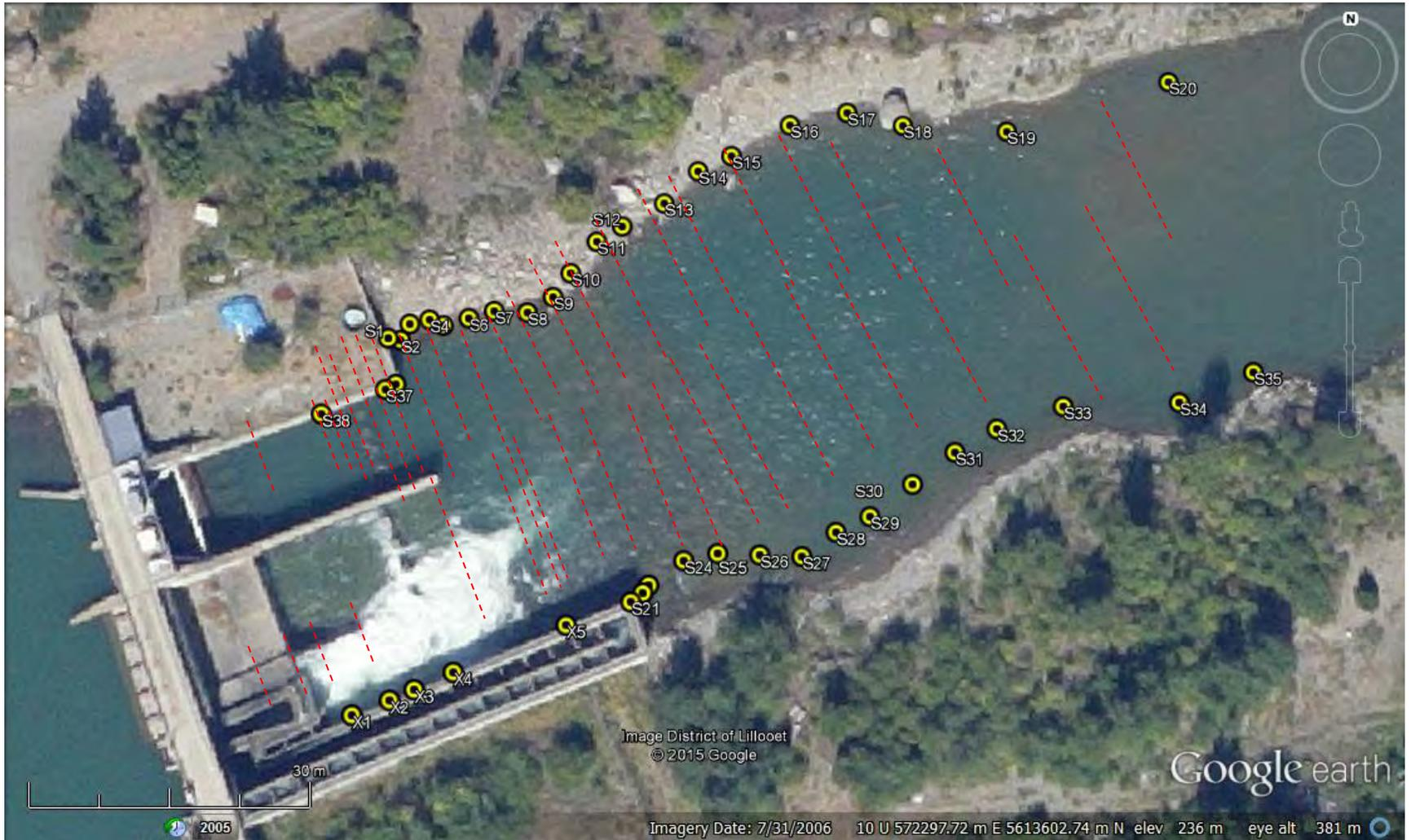
Figure 5. ADCP measurement sections in 2014.
