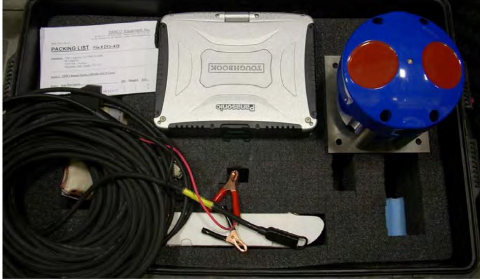
Figure 3. Teledyne RDI ChannelMaster H-ADCP 1200 kHz.
