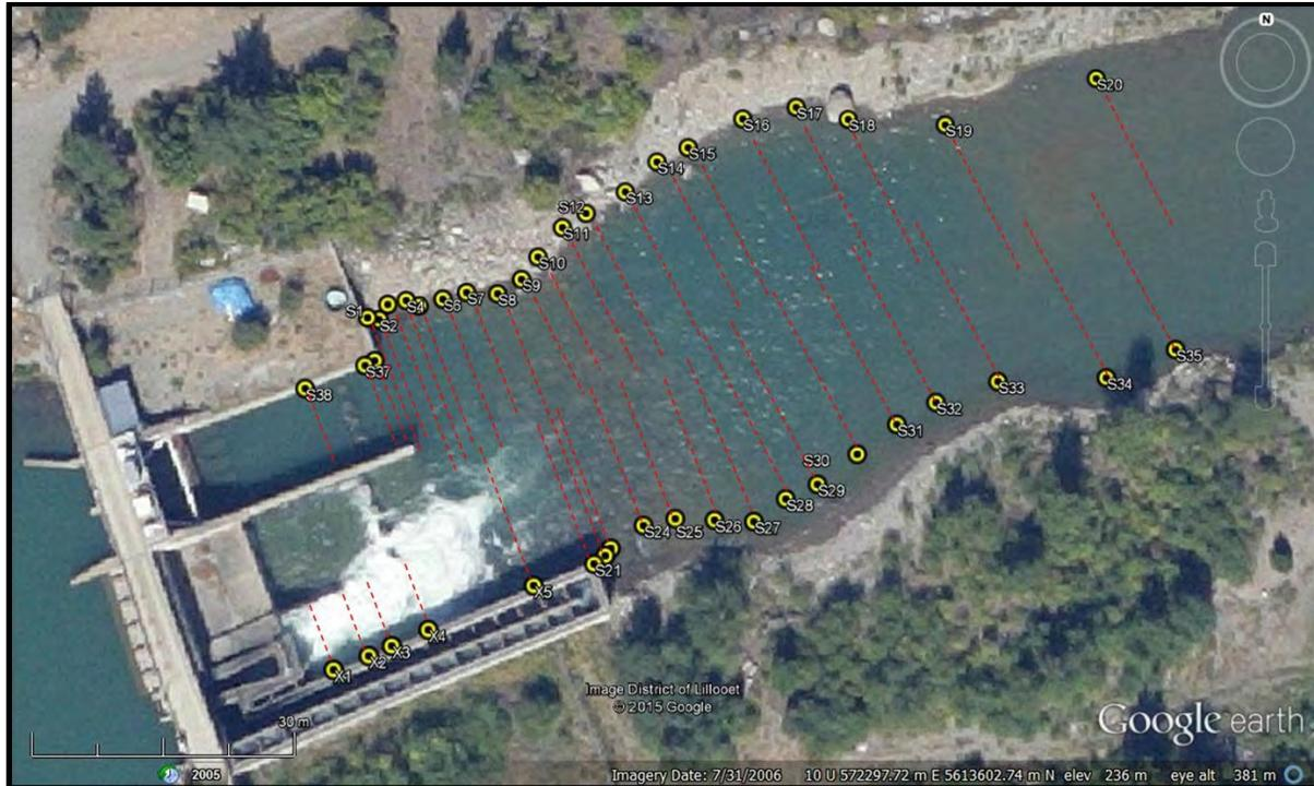
**Figure 2-2: Acoustic Doppler Current Profiler measurement transects in the Seton Dam tailrace (S1-S38) and at the fishway entrance (X1-X5) in 2014**
