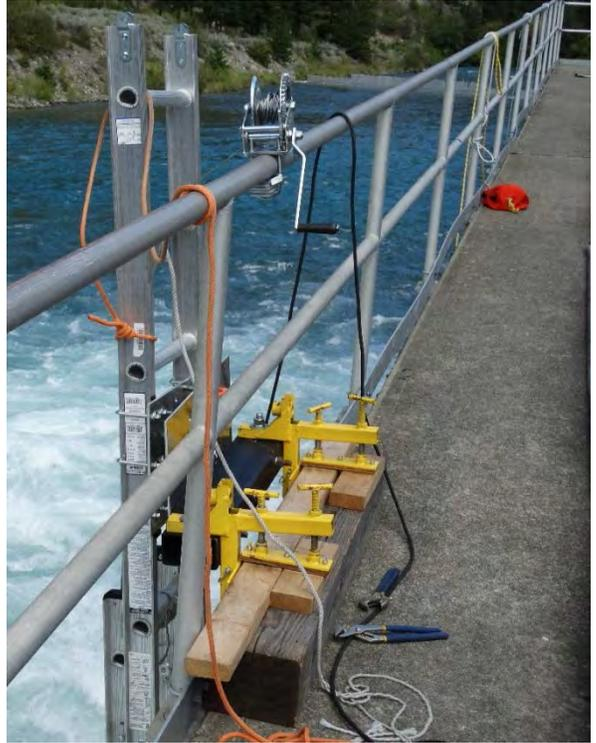
**Figure 7. ADCP frame for measurements in the dam tailrace.**
