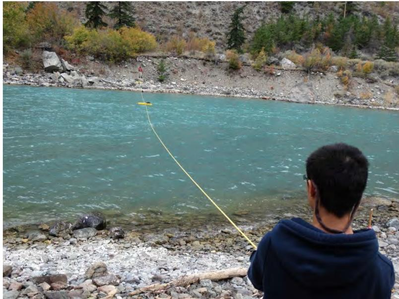
**Figure 9. Towing the Sontek ADCP across the river to measure bathymetry.**
