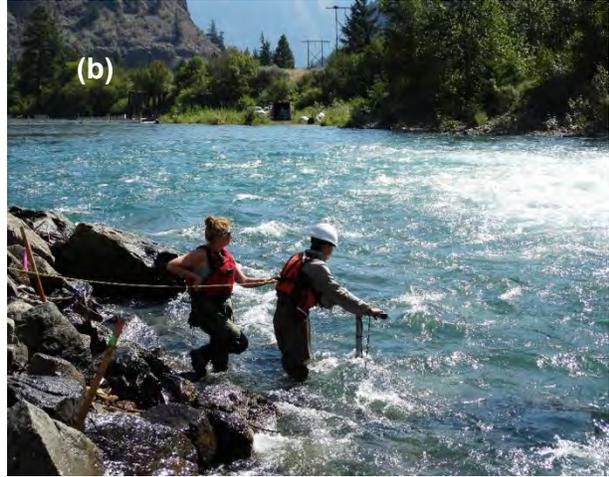
**Figure 6. (a) ADCP “T”-shaped frame for measurements in the Seton River. (b) H-ADCP during measurement.**
