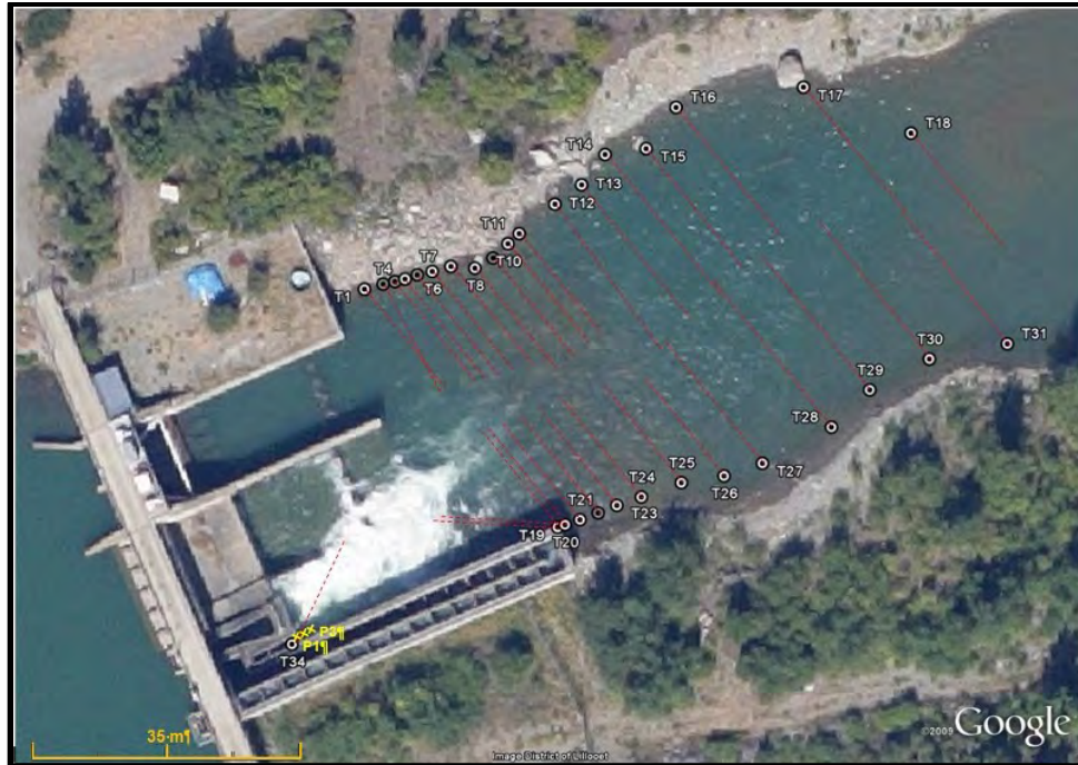
Figure 2-2: Acoustic Doppler Current Profiler measurement transects in the Seton Dam tailrace (T1-T34) and at the fishway entrance (P1-P3)
