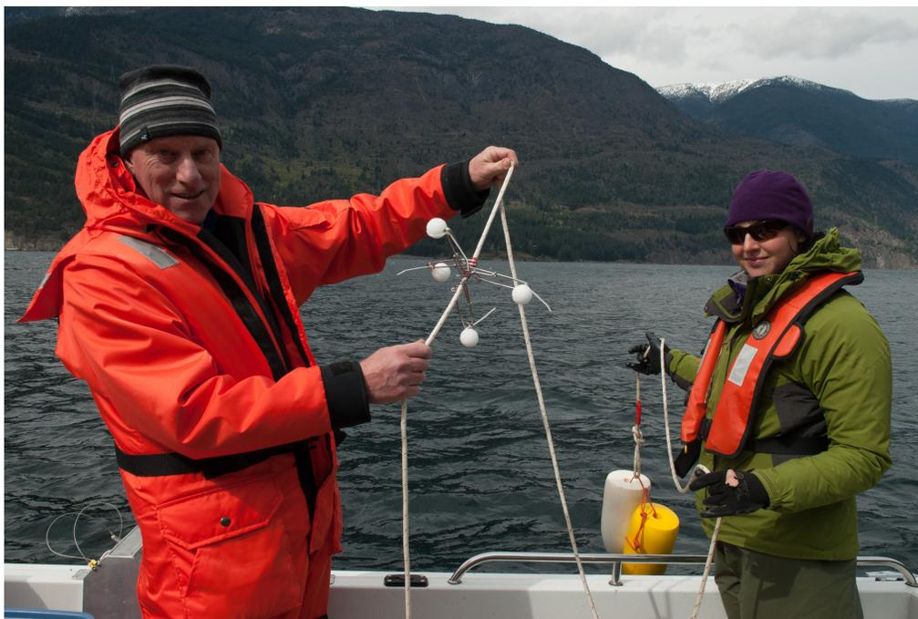
Figure 7. Styrofoam array used to represent periphyton growth on stable substrata.
