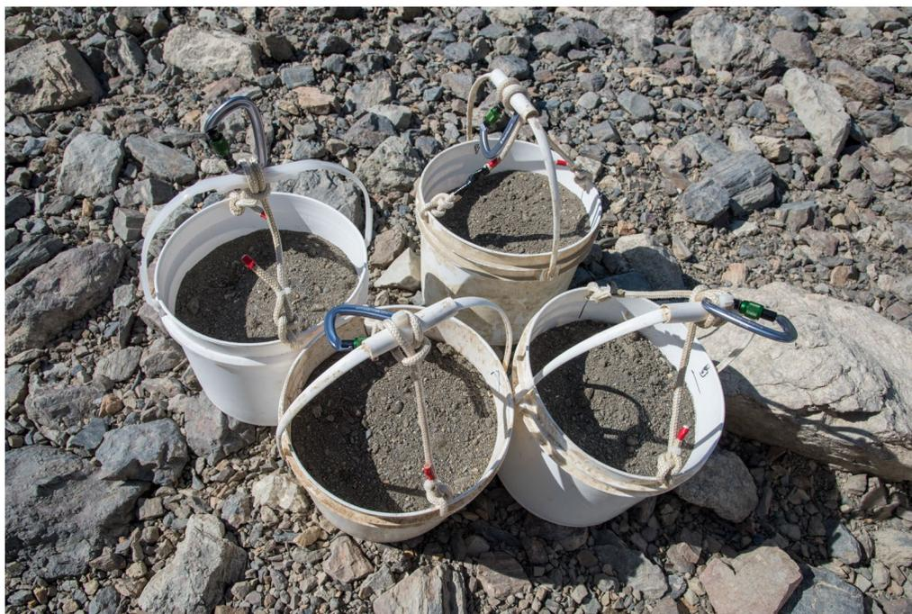
Figure 8. Sand pails used to host periphyton growth on sand in Carpenter Reservoir. Rigging on the pail handles was used to clip the pails onto lines of fixed length that were suspended from a boom. This arrangement provided a range of pail depths extending from close to the water surface to the bottom of the euphotic zone.
