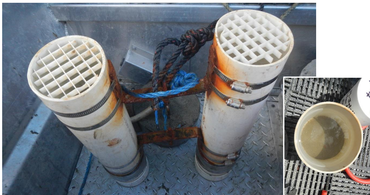
Photo 2.1 Sedimentation sampler deployed year-round in Seton and Anderson lakes since Year 4 (2016). The removable sampling cups from which the sediment samples were collected is also shown (inset).
