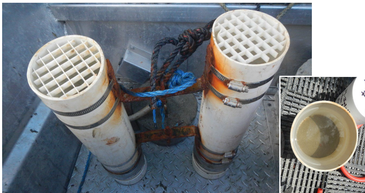
Photo 2.1 Sedimentation sampler deployed year-round in Seton and Anderson lakes since Year 4 (2016). The sampling cup from which the sediment sample was collected is shown (inset).
