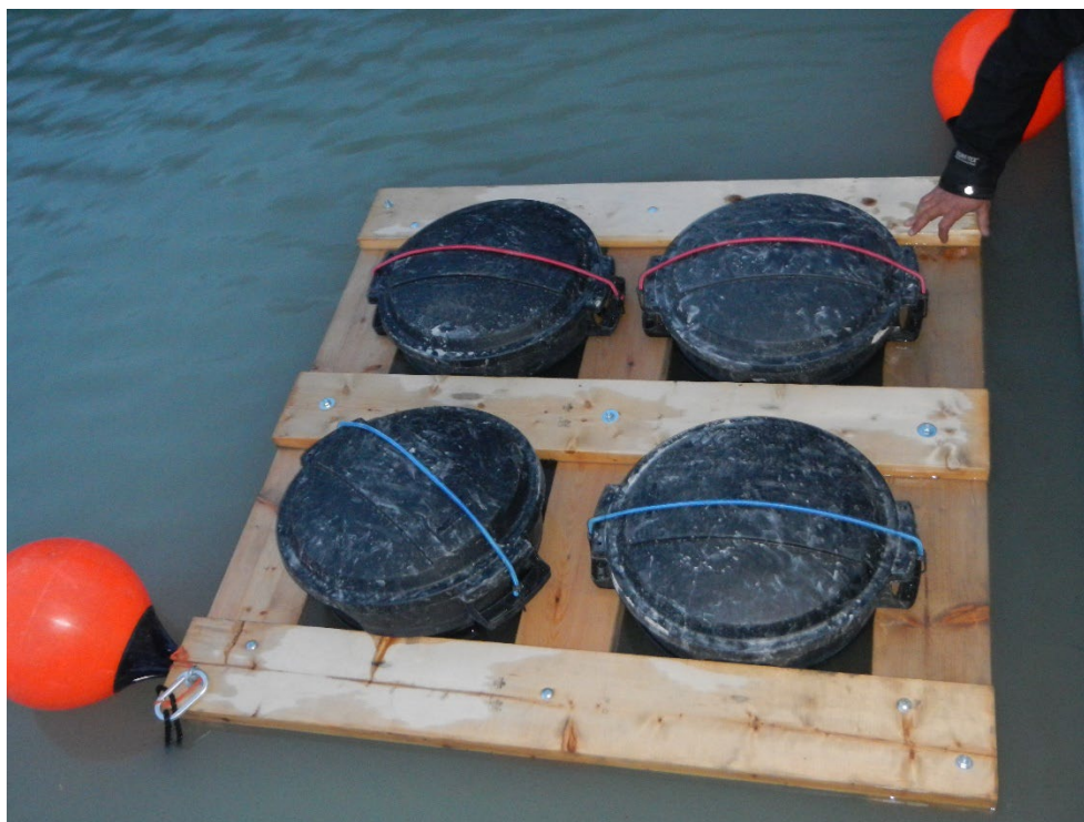
Photo 2.1 Floating fish-holding tank used during the Years 5-8 (2017–2020) Downton Reservoir fish population index surveys to assess the incidence of fish mortality and tag loss 24-hours post-capture.
