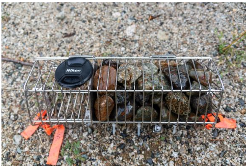
Photo 2.3 Basket sampler before installation in the Lower Bridge River. Baskets used in 2020 were longer than those from previous years. To ensure consistency of data among years, a baffle was installed in each basket so that it contained the same volume of packed stones as previous samplers.
