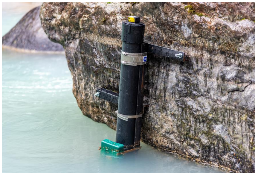
Photo 2.1 The turbidity logger housing installed at Rkm 36.8. The green shield was installed over the sensor to limit exposure to sunlight that can produce faulty readings.
