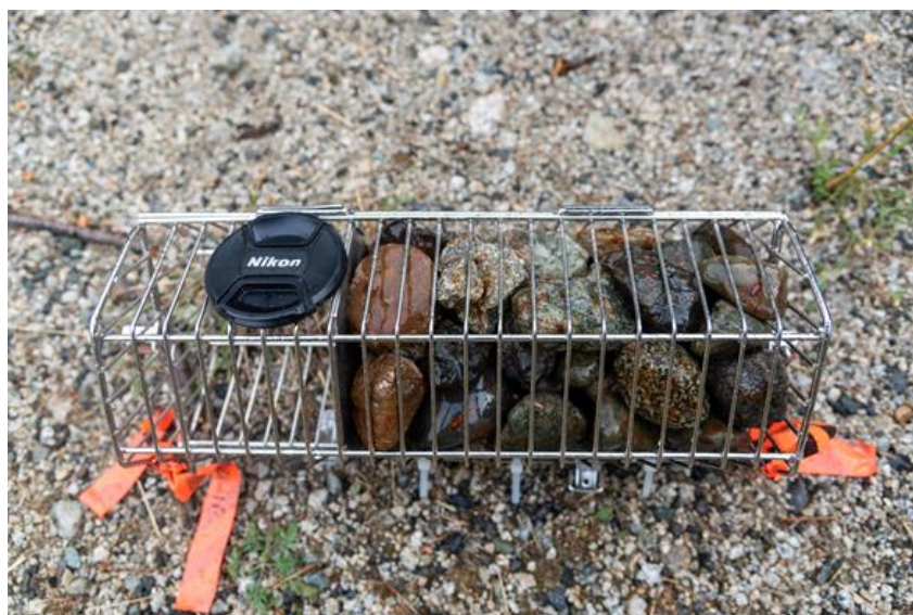
Photo 2.3 Image of a basket sampler before installation in the Lower Bridge River. Baskets used in 2020 and 2021 were longer than those from previous years. To ensure consistency of data among years, a baffle was installed in each basket to contain the same volume of packed stones as in previous years.
