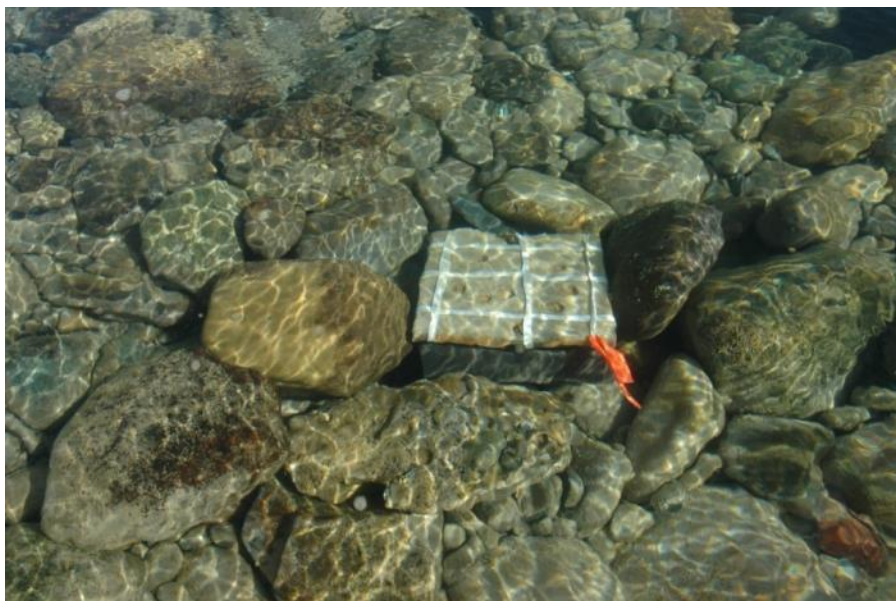
Photo 2.2 Image of an installed periphyton plate.
