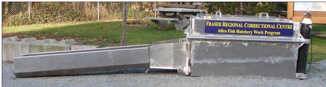
**Figure 5 Sockeye transport tank with release slide connected, January 2010**
