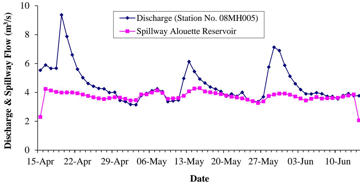
Figure 4. Daily discharge ( $\text{m}^3/\text{s}$ ) at Water Survey of Canada Station No. 08MH005 and spillway flows from the Alouette Reservoir (15 April–15 June 2013). The WSC station is located on the mainstem South Alouette River at the 232<sup>nd</sup> Street bridge (discharge data from Water Survey of Canada website: <http://www.ec.gc.ca/rhc-wsc/>).
