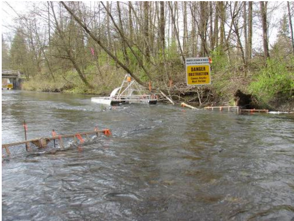
Figure 2.4. Typical rotary screw trap placement 14 April – 14 June. Note the use of screen panels and sandbags to concentrate flows and enhance trap efficiency.
