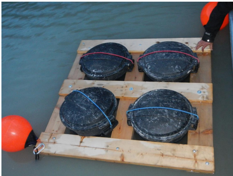
Photo 2.1 Floating fish-holding tank used during the 2017 & 2018 Downton Reservoir fish population index survey to assess the incidence of fish mortality and tag loss 24-hours post-capture.
