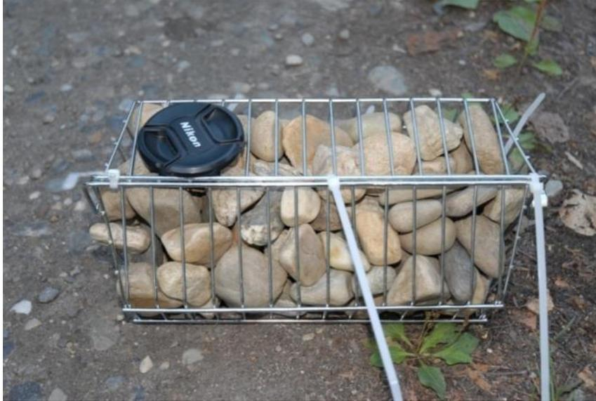
**Photo 2.2 Basket sampler before installation in the Lower Bridge River.**
