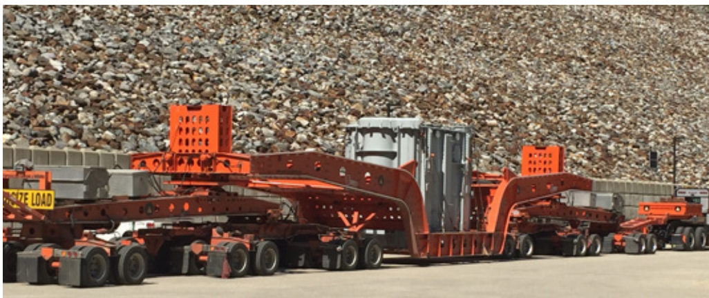
A new transformer – close to 105 tonnes – delivered to Mica Generating Station.
