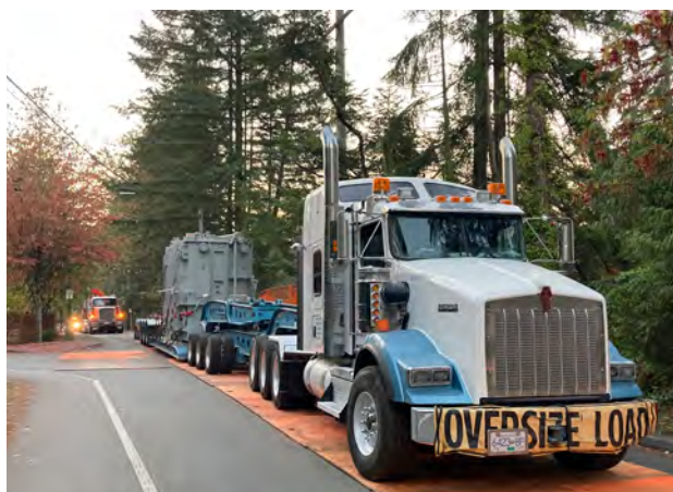
The delivery truck carrying the transformer. The specialized truck and trailer has 13 axles and 50 tires to spread out the load and reduce contact pressure on roads and bridges. The truck carried the transformers – one at a time – from the port in Everett, Washington to a drop-off point in North Vancouver.
