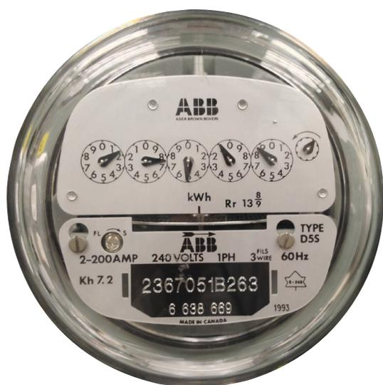
The faster the disk turns, the more energy is being consumed. You can estimate how much energy would be consumed in an hour by counting the number of disk revolutions in two minutes.
