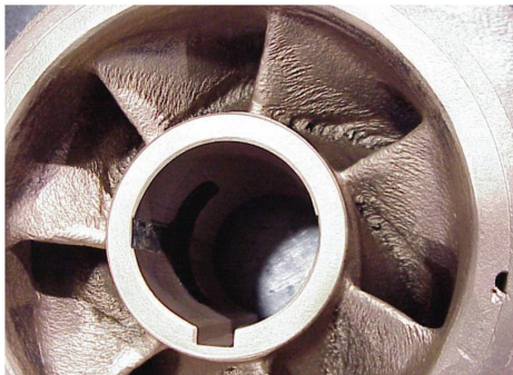
Figure 14: Extreme Example of Impeller Cavitation and Corrosion (Photo courtesy of the Association for Iron & Steel Technology)
