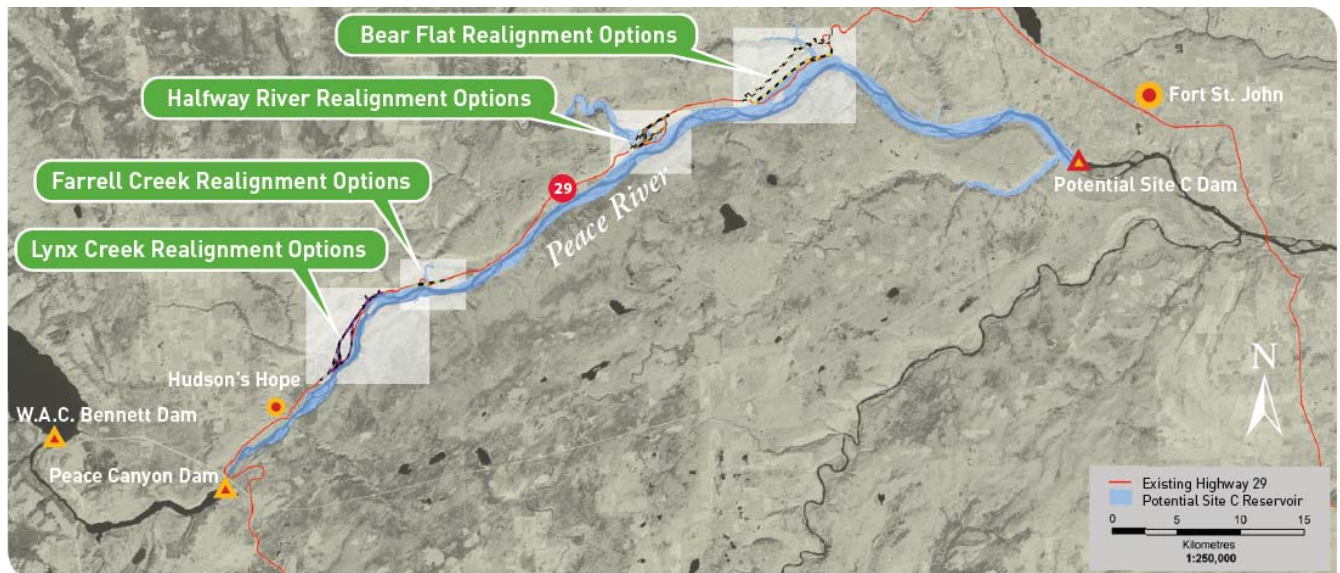
Highway 29 Realignment Segments
