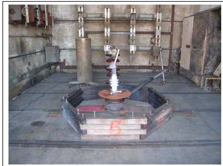
Figure 3 – Test Set-Up for Short Circuit Tests
