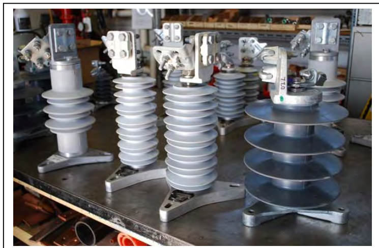
Figure 1 – Station Class Arresters Used During the Tests
