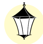
Bad— Waste light goes up and sideways
