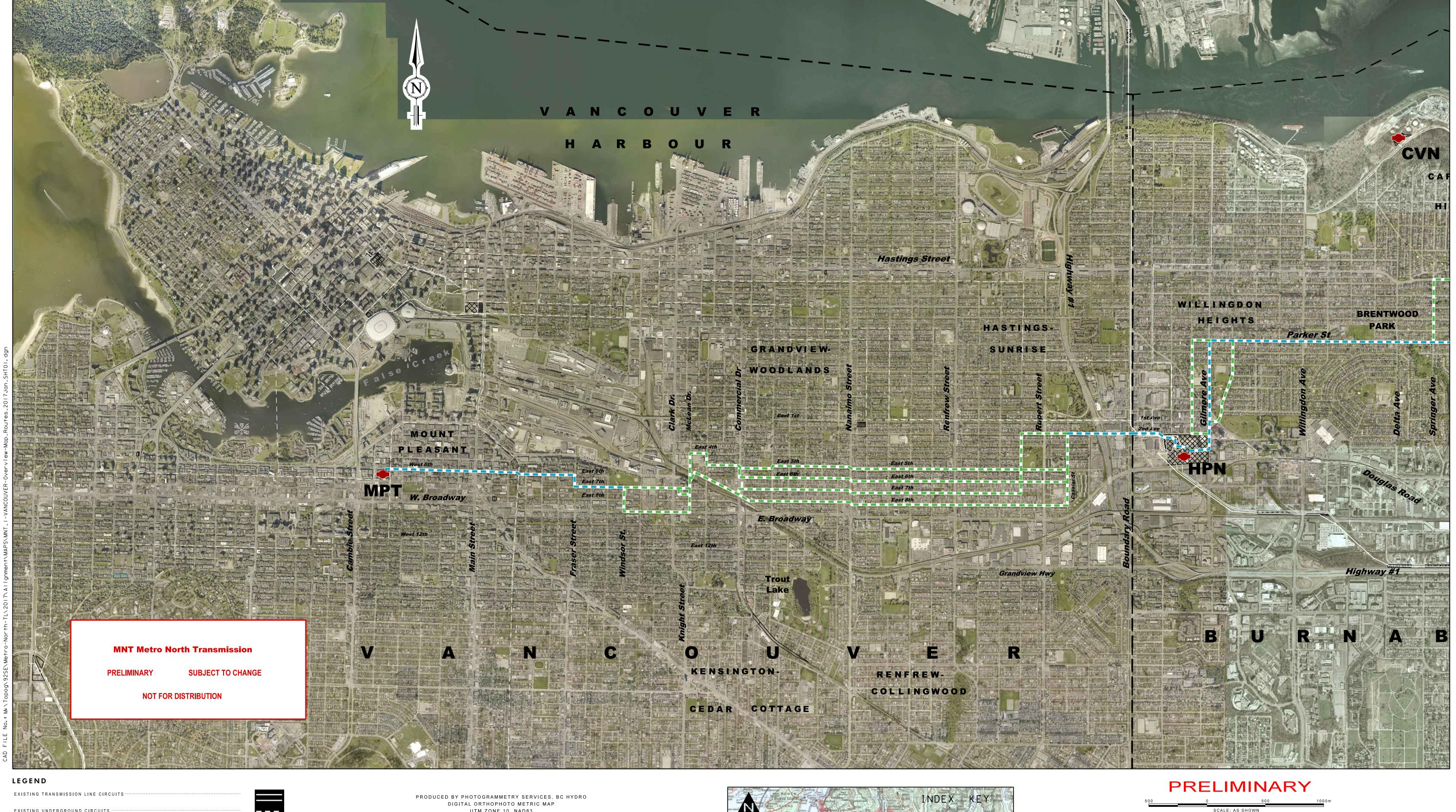
EXISTING UNDERGROUND CIRCUITS ... BC HYDRO FEE OWNED… LEADING U/G ROUTES · LEADING O/H ROUTES ·· ALTERNATE ROUTES (UG and OH). SUBSTATION ... MUNICIPAL BOUNDARIES ...
