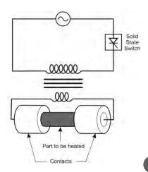
physically make contact with the product being heated. See diagram above. For food products, the sauce or gravy is the component that conducts the electric current, and the process is sometimes called "ohmic heating." The resistance (R) of the product to the flow of current (I) passing through it generates the I²R heating power. Low frequency current (60 Hz) heats the part throughout. High frequency current (400 kHz) tends to heat only the surface of the part.
