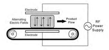
This characteristic is useful for speeding up the heating and drying of adhesives in the production of laminated products,
