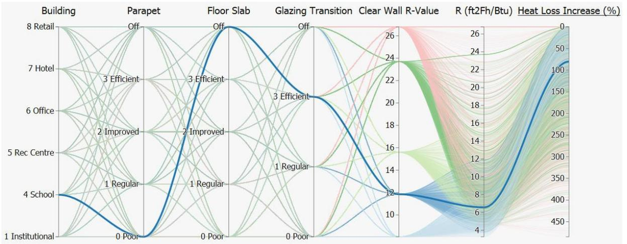
**Figure 2 – Parametric Analysis of Base Building U-Value Impacted by Thermal Bridging**
