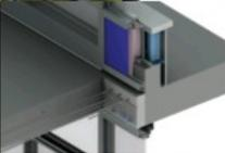
Improved  | <b>Thermally broken and intermittent structural connections</b><br>Examples: structural thermal breaks, stand-off shelf angles.                                      | 0.20                 | 0.35     |
