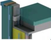
Efficient | <b>Roof and Wall Insulation Meet at the Roof Deck</b><br>Examples: structural thermal break at roof deck, wood-frame parapet.                                             | 0.12                                | 0.2                           |
