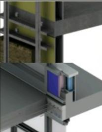
Efficient | <b>Fully insulated with only small conductive bypasses</b><br>Examples: exterior insulated wall and floor slab.                                                      | 0.12                 | 0.2      |
