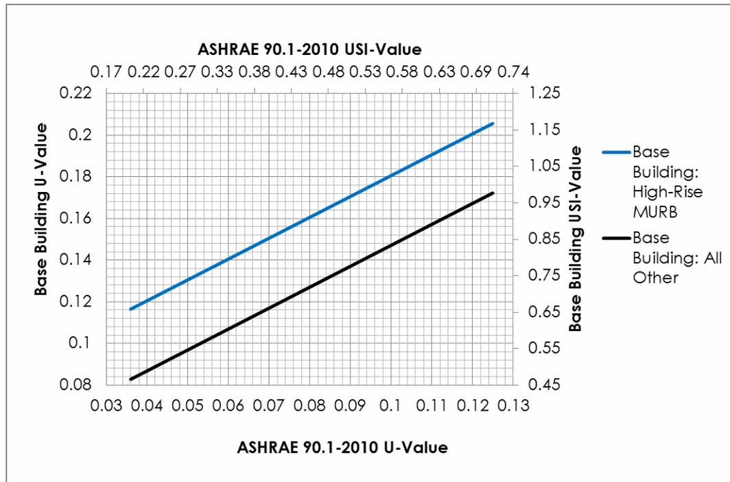
**Figure 6** – Effective U-value Accounting for Linear Heat Losses for Varying Clear Wall U-values
