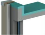
Improved  | <b>Fully Insulated Parapet</b><br>Examples: insulation wraps around the parapet to the same insulation level as the roof and wall.                                        | 0.17                                | 0.3                           |
