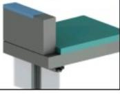
Poor      | <b>Un-insulated and major conductive bypasses</b><br>Examples: exposed parapet and roof deck.                                                                             | 0.46                                | 0.8                           |
