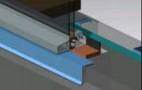
Poor      | <b>Un-insulated and conductive bypasses</b><br>Examples: metal closures connected to structural framing. Un-insulated concrete opening (wall insulation ends at edge of opening).         | 0.29                 | 0.5      |
