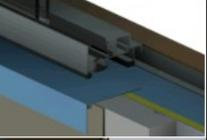
Regular   | <b>Misaligned glazing and minor conductive bypasses</b><br>Examples: wall insulation is not continuous to thermal break and framing bypasses the thermal insulation at glazing interface. | 0.20                 | 0.35     |
