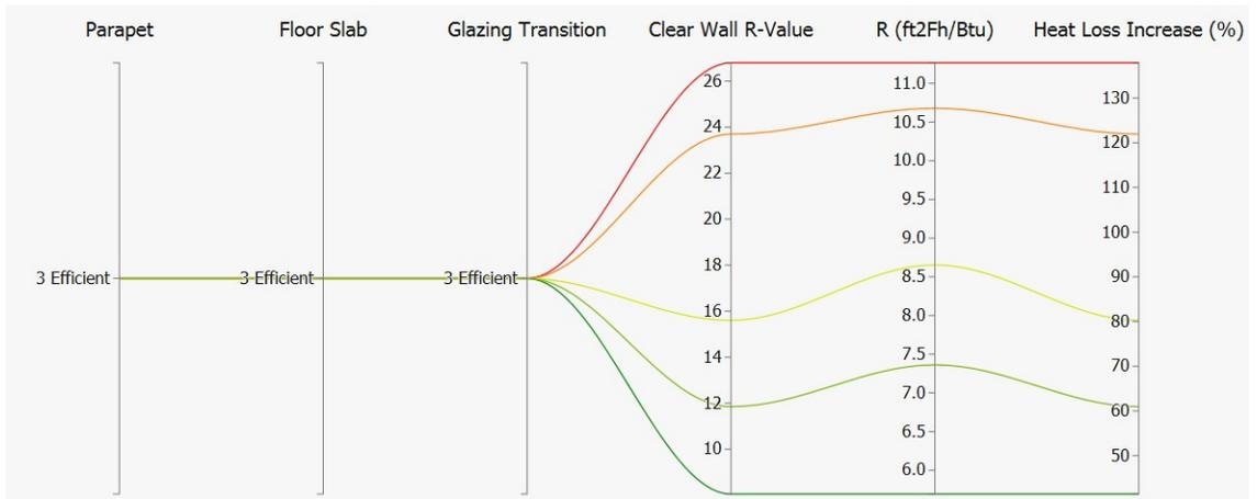
**Figure 4 – Impact of Clear Wall on Heat Loss Increase over Base Building**
