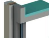
Regular   | <b>Under-insulated Parapets</b><br>Examples: concrete parapet is partially insulated (less than roof insulation), insulated steel framed parapet, concrete block parapet. | 0.26                                | 0.45                          |
