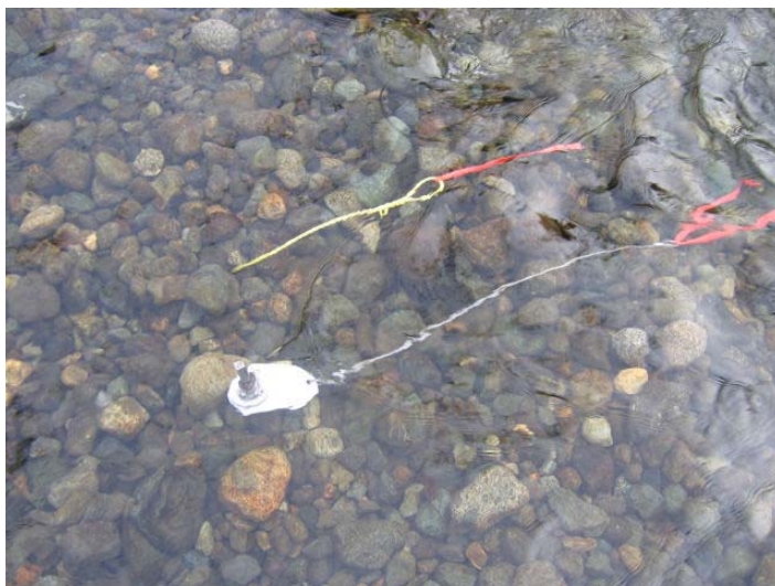
Photo 3. Paired Jordan and pipe incubators (showing top plate) after burying in the gravel.
