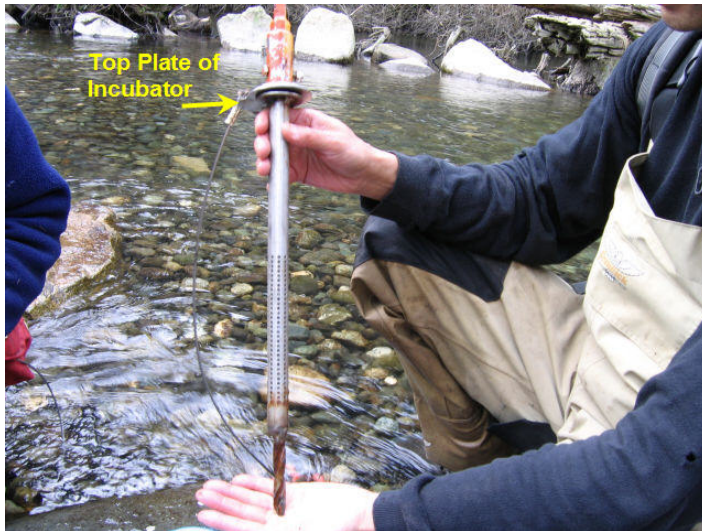
Photo 1. Pipe incubator used in Bull Island side-channel to test incubation success. Top plate indicates depth at which incubator is buried.
