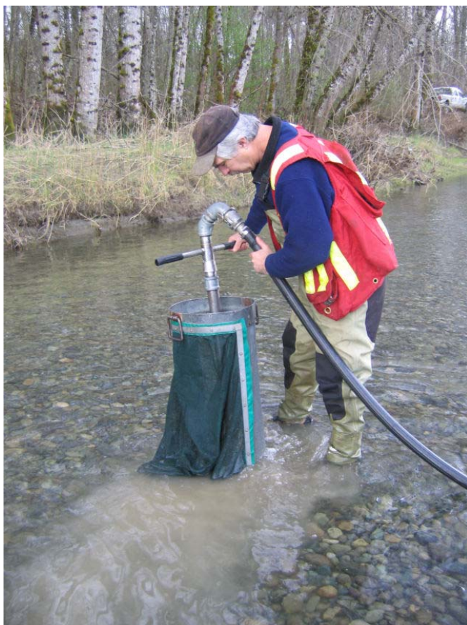
Photo 5. Hydraulic sampling - nozzle is inserted into gravel forcing eggs/alevins to surface in catch net.
