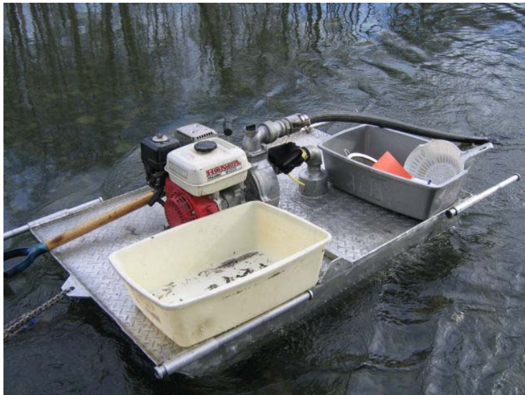
Photo 4. Hydraulic sampling equipment used to assess embryo survival of natural spawn in Bull Island side-channel, December 9, 2005.
