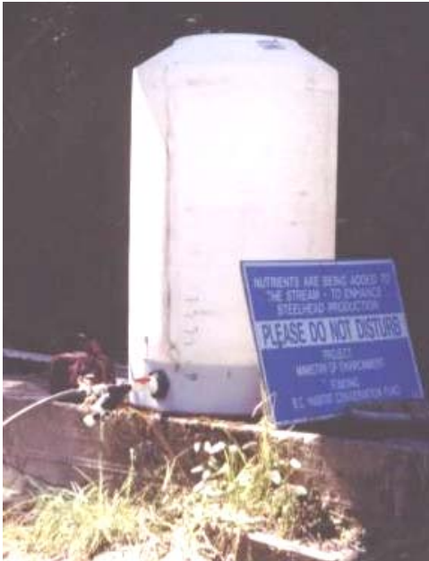
Figure 2. The fish screen tank site under the Salmon River ML Bridge, 2003. Tank capacity is 624 L.
