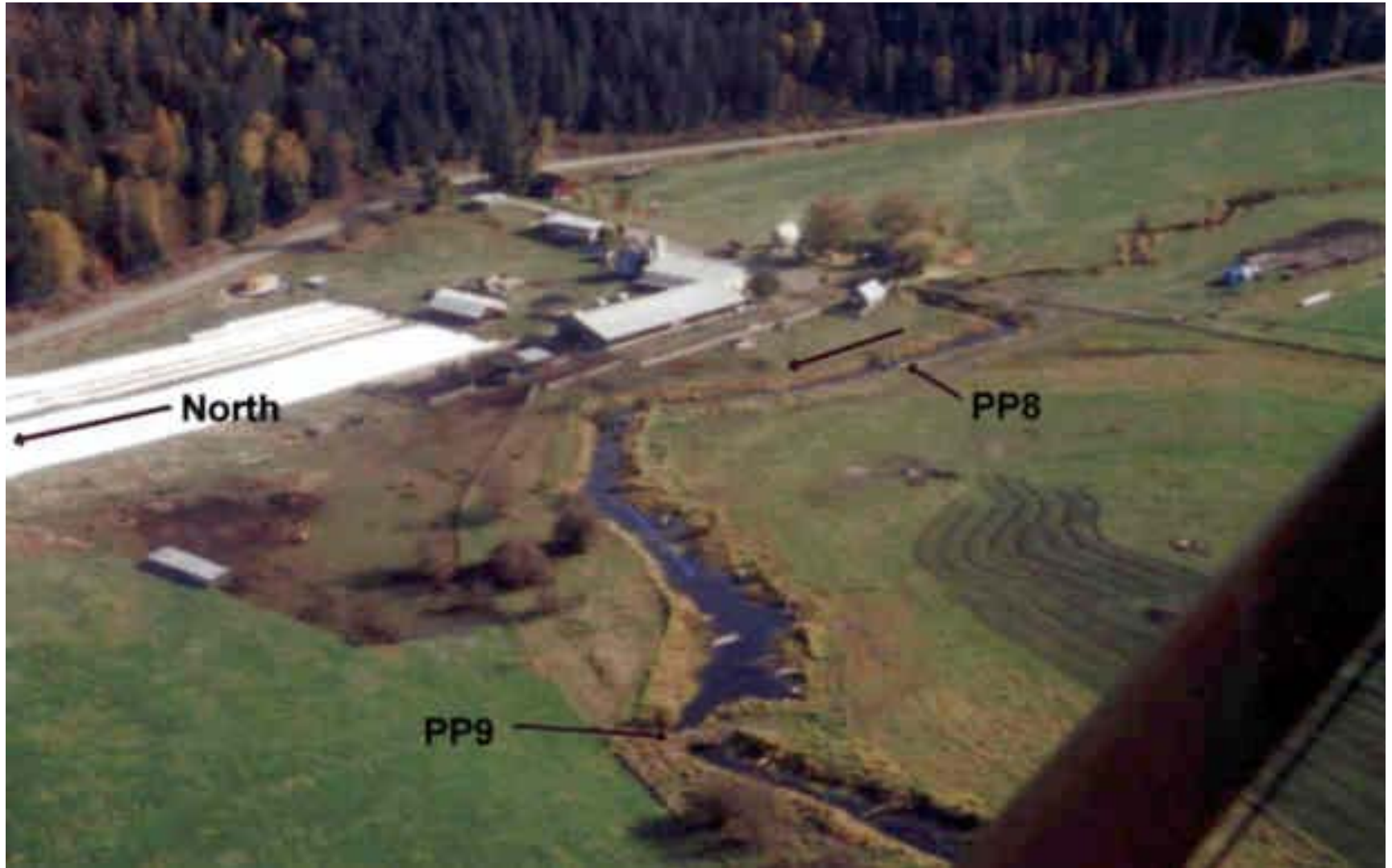
Air photo 4: The channel is wider on the lower section as it picks up groundwater.
