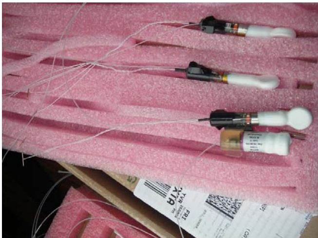
Photo 1. Three Lotek Electromyogram (EMG) transmitters and one Conventional MCTF 3A transmitter with temperature loggers attached.
