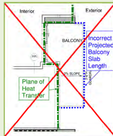
Incorrect Project Balcony Slab Length for Calculations
